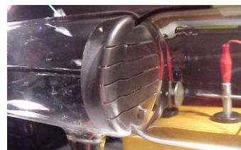
The cathode possesses slits or holes
