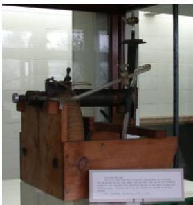
1913, Thomson's parabola spectrograph (Museum at the Cavendish Laboratory)
