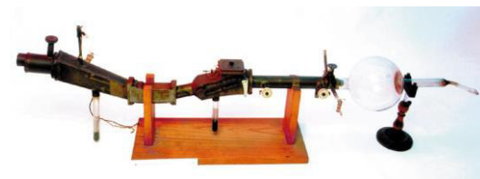
1937: Aston's third mass spectrograph (Museum of the Cavendish Laboratory) Resolution: 2000
