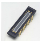
1024-element CMOS photodiode array (Hamamatsu)
